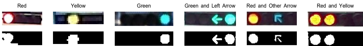
Fig. 3. Results of the signal synthetic segmentation dataset showing traffic light ROIs and their pseudo masks
